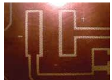
Figure 2. Etched copper circuit trace on thermal dielectric & actual etched circuit; 60X.
