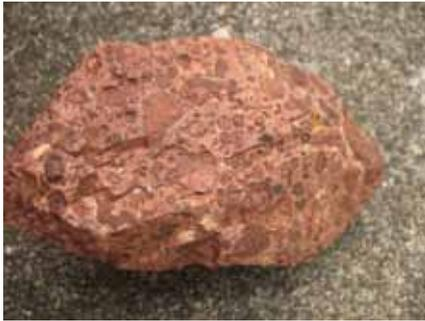
Figure 1. Bauxite raw material: The basis for the production of aluminum and ceramic. Source: Geological collection, University of Tübingen, thanks to Dr. Udo Neumann
