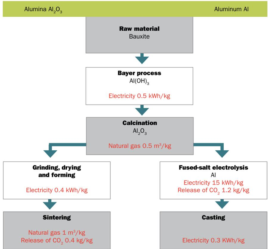
Figure 2. Overview of energy-relevant processing methods. Note: Several energy sources are used in this process. To increase clarity, all numerical values in this article have been simplified and rounded.
