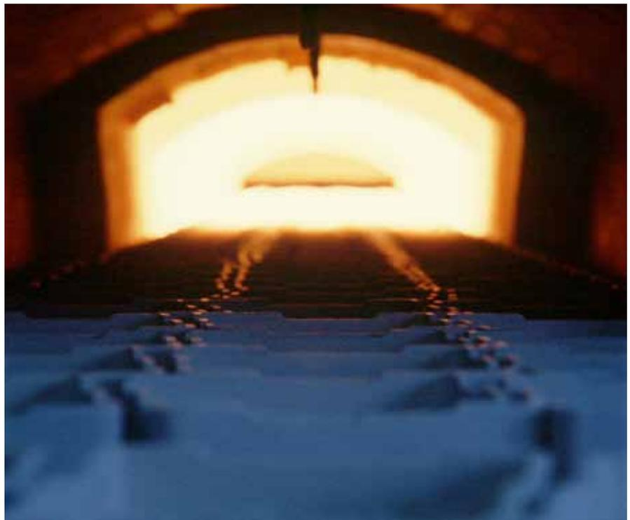
Formed ceramic parts undergo heat treatment below the melting temperature; alumina Al<sub>2</sub>O<sub>3</sub> e.g. at 1300-1600 °C (air). Sintering uses the most energy of all process steps in the production of ceramic, yet the amount of CO<sub>2</sub> released is only half the amount released in aluminum production.
