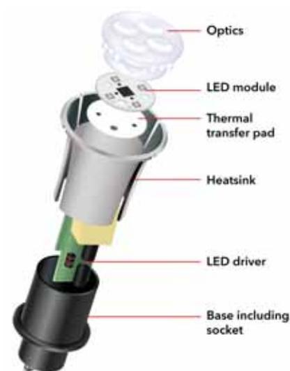
Figure 1. LED lamp construction: terminals, heatsink, housing, lens, control electronics, LED module
